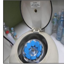
Figure 27. Placing the centrifuge tubes into the centrifuge
