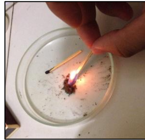
Figure 50. Evaluating the flammability of Iron oxide Microparticles.
