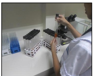
Figure 58. Testing the TFC of the wastewater
