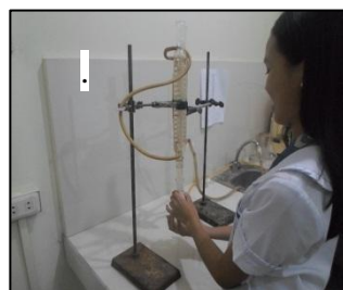
Figure 56. Testing the COD of the wastewater
