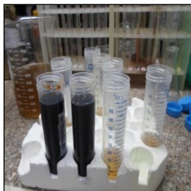
Figure 24. Adding 40 ml of ferric chloride solution into the test tube
