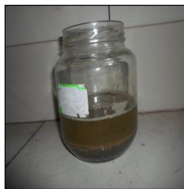
Figure 42. Sand soaked in an 8% Nitric acid solution
