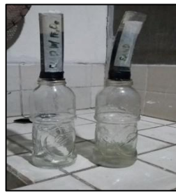
Figure 38. The Sand with Iron oxide microparticles filter and the sand filter
