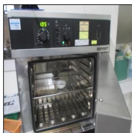
Figure 33. Placing the evaporating dish in the oven
