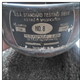
Figure 40. Sieve with holes between 0.85 and 2.36 mm
