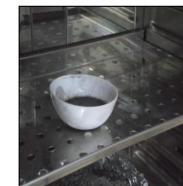
Figure 35. The evaporating dish inside the oven for 5 hours
