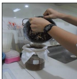
Figure 20. Filtering the mixture using a cloth
