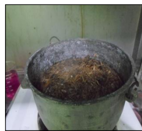
Figure 18. Boiling of 50 grams bagasse in 100 mL distilled water for 10 minutes
