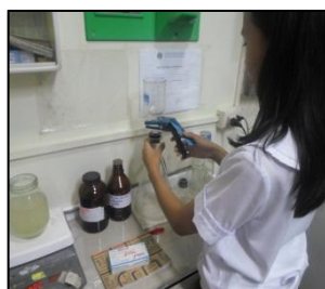
Figure 58. Testing the TSS of the wastewater
