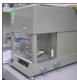
Figure 16. Measuring 50 grams of bagasse
