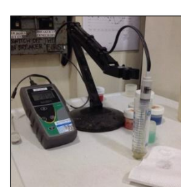
Figure 47. Evaluating the pH level of the Iron oxide
