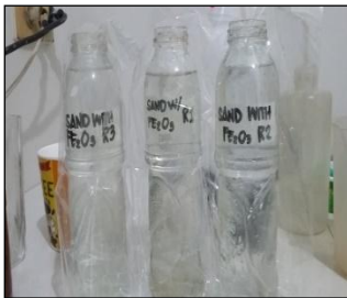
Figure 52. The wastewater samples after being filtered using the biosand composite with iron oxide microparticles
