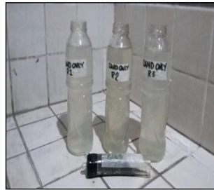
Figure 53. The wastewater samples after being filtered using sand only.
