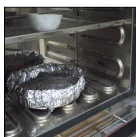
Figure 45. Drying the sand in the oven
