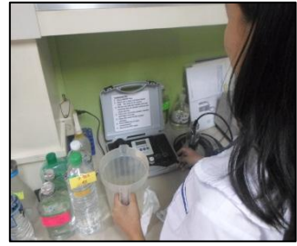
Figure 55. Testing the turbidity of the wastewater
