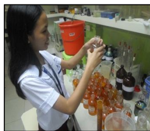
Figure 57. Testing the DO of the wastewater
