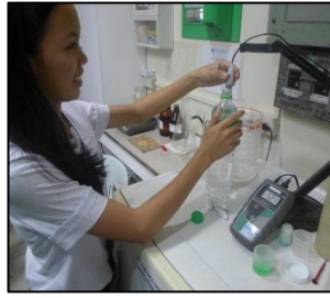
Figure 54. Testing the pH of the wastewater
