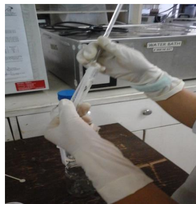
Figure 36. Collecting the solid particles after the centrifuge process (Photo taken by :CJP ,Lijayan)
