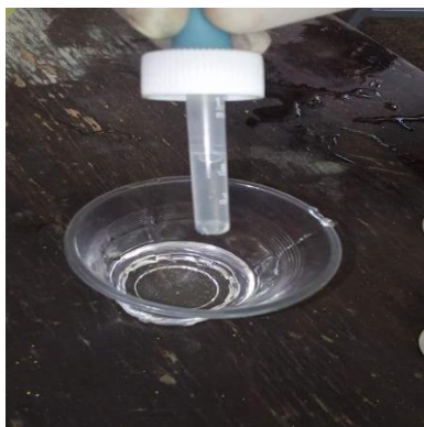
Figure 50. Dropping the 0.25ml hardener on the container (Photo taken by : TP , Advincula)
