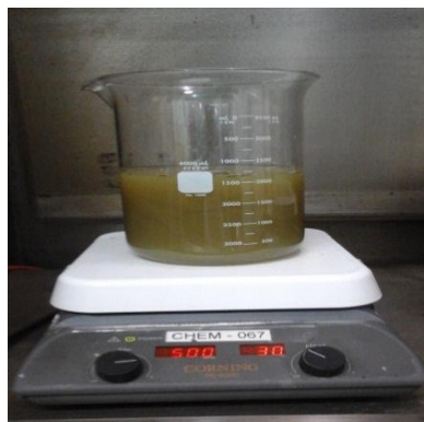
Figure 13. The chicken feather and sodium sulfide solution after 6 hours of stirring (Photo taken by: TP, Advincula)
