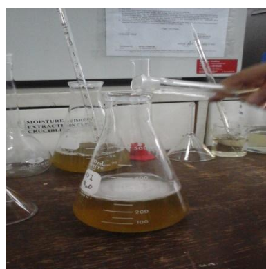
Figure 23. Ammonium sulfate was added drop wise and was shook after every drop (Photo taken by :CJP ,Lijayan)
