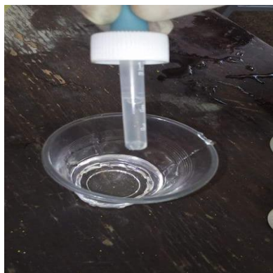
Figure 49. Dropping corresponding amount of keratin solution into containers (Photo taken by : TP , Advincula)
