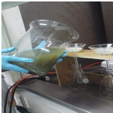
Figure 14. Filtering of the chicken feather mixed with sodium sulfide solution (Photo taken by: TP, Advincula)
