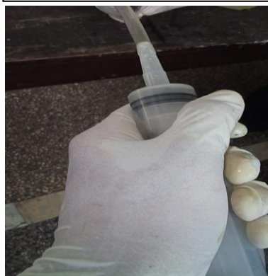
Figure 52. Inserting the of the syringe to the polytube (Photo taken by : TP , Advincula)
