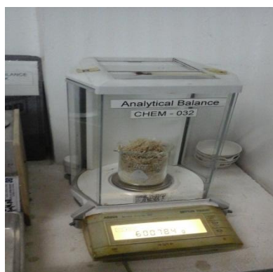
Figure 10. Weighing of the shredded chicken feathers (Photo taken by: TP, Advincula)
