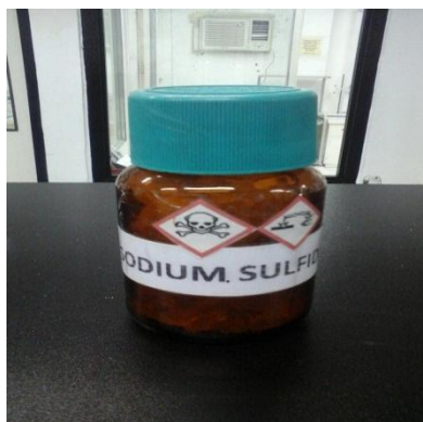
Figure 5. The chemicals used are: Sodium Sulfide to dissolve the chicken feathers and Ammonium Sulfate for the precipitation process (Photo taken by: TP, Advincula)
