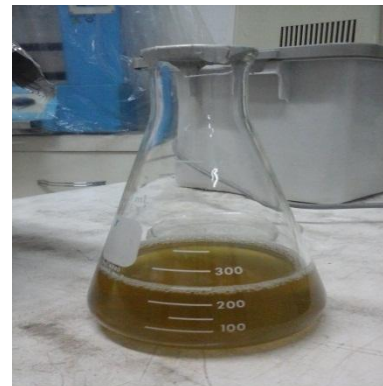
Figure 15 The filtered chicken feather and sodium sulfide solution in the Erlenmeyer flask. (Photo taken by: TP, Advincula)
