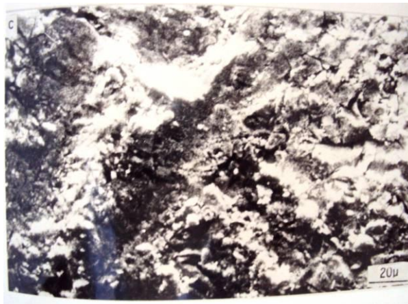
Figure 5 (20 \mu ). Scanning electron microscope (S.E.M.), surface texture photomicrograph of DSC slag showing the very rough (deep pores) exposed weathered surface with whitish calcium silicate hydrate (CSH) coatings and infillings.
