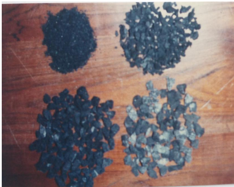
Figure 3. Photograph of DSC slag showing consistent physical shape and surface texture characteristics even on consistent grading to the fine, sand size.
