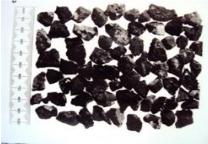
Figure 2. Photograph of a typical Jaw crusher produced <math>< 14.00\text{mm}</math> - 10mm DSC slag showing consistent angular and irregular to sub-rounded shape and rough, vesicular surface texture features with whitish infillings and coatings. The angularity and vesicularity, provides good macadam/tar binding face as an aggregate in the construction and as railway ballast in the transport industry.
